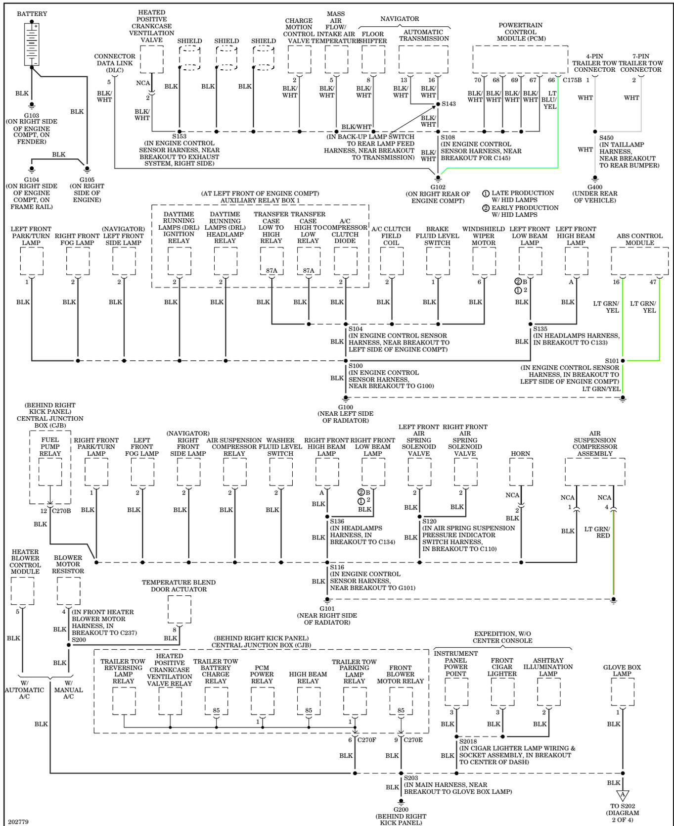
Ground Distribution Wiring Diagram (1 of 4)
